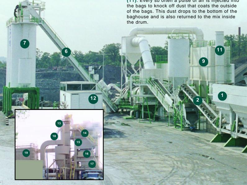
The entire operation is controlled and monitored by a computer, or a **programmable controller** (12), which make sure the system is performing properly and warns the operator of any failure.
